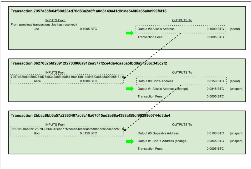
Figure 2-4. A chain of transactions, where the output of one transaction is the input of the next transaction
